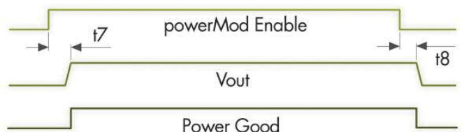
Output powerMod Signals
