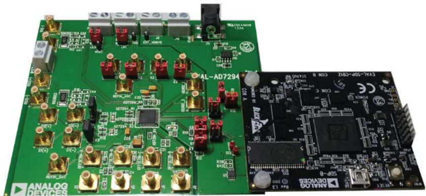
Figure 1. Universal Evaluation Board Connected to the SDP-B Board
