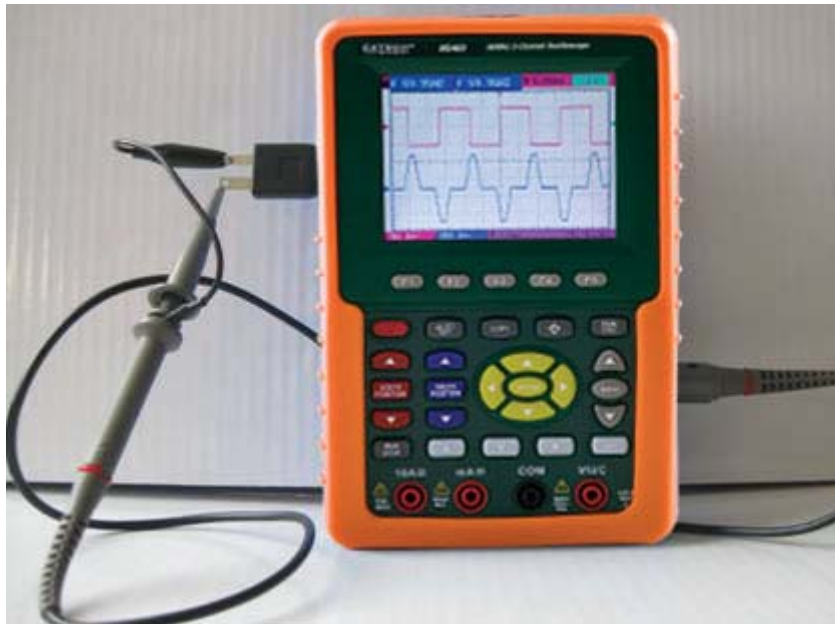
Fig 39: Square-wave test signal
