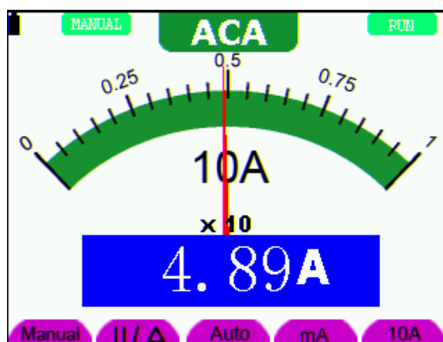
Figure 11: AC Current Measurement for 10A
