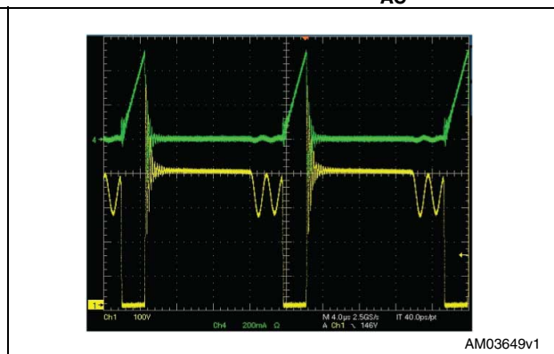
Figure 8. Drain current and voltage at maximum load 230 V AC
