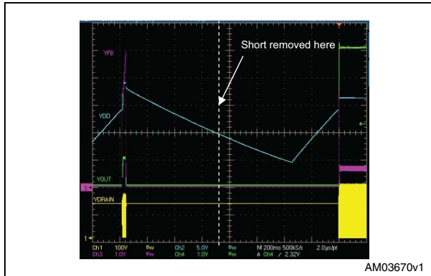
Figure 30. OLP: steady-state, short removal and restart
