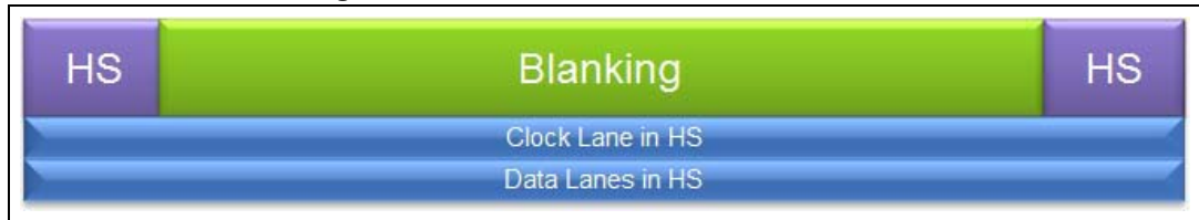
Figure 141. Clock lane and Data lane in HS
