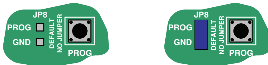
a) No Jumper: FPGA Operational (default)
