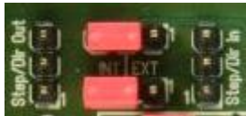
Figure 3.7 Jumper setting for TMC4210 selection.
