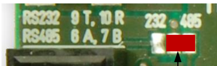
Solder bridge for RS485
