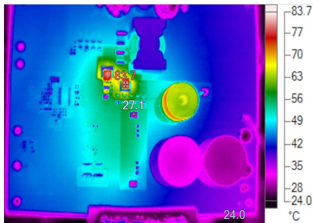
Figure 6. Thermal Image, 12V Input to 240V Output at 0.7A, No Air Flow, No Heat Sink, Top Side.
