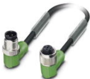
Sensor/actuator cable, 4-position, PUR halogen-free, black-gray RAL 7021, Plug angled M12, A-coded, on Socket angled M12, A-coded, cable length: 0.3 m
