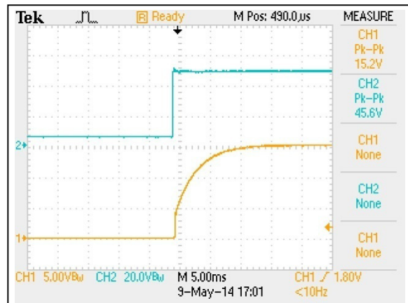
Figure 97: AEE02C36-L Output Voltage Startup Characteristic by Vin Vin = 48Vdc Load: Io = 2.67A Ch1: Vo Ch2: Vin
