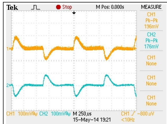
Figure 49: AEE01BB18-L Transient Response Vin = 24Vdc Load: Io = 100% to 75% load change Ch 1: Vo1 Ch 2: Vo2
