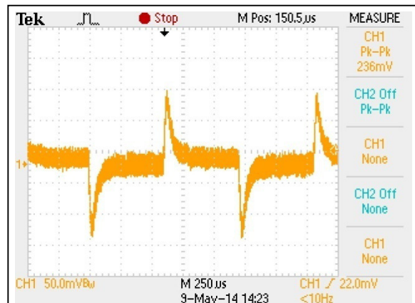
Figure 40: AEE01H18-L Transient Response Vin = 24Vdc Load: Io = 100% to 75% load change Ch 1: Vo
