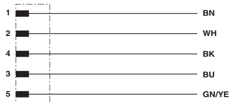
Contact assignment of the M12 plug
