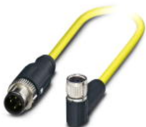
Sensor/Actuator cable, 4-position, PVC, yellow, shielded, Plug straight M12 SPEEDCON, A-coded, on Socket angled M8, Cable length: 0.5 m
