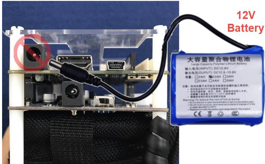
Figure 3-15 Connect Power JACK to 12V Battery is banned
