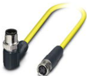
Sensor/Actuator cable, 3-position, PVC, yellow, shielded, Plug angled M12 SPEEDCON, A-coded, on Socket straight M8, Cable length: 1.5 m
