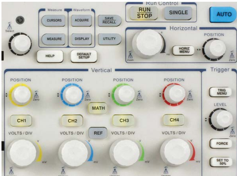
Figure 11 - Control Buttons (4CH model shown)
