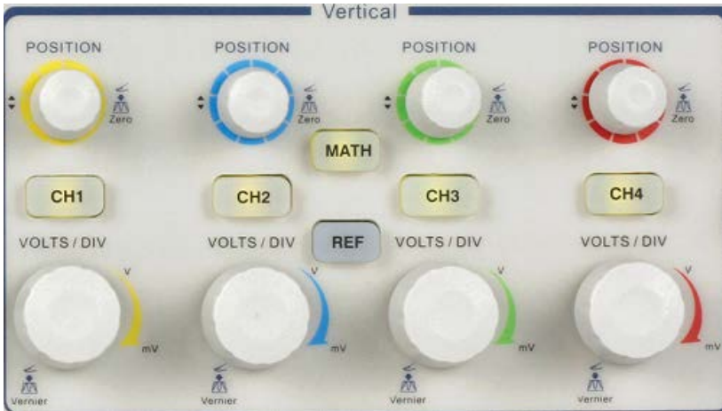
Figure 15 - Vertical System Controls
