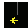
Pre/Post-Trigger – appears at corner of grid when trigger point is no-longer visible.
