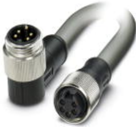
Bus system cable, DeviceNet, 5-position, PVC, Gray RAL 7001, Plug angled 7/8"-16UNF, on Socket straight 7/8"-16UNF, Cable length: 1 m
