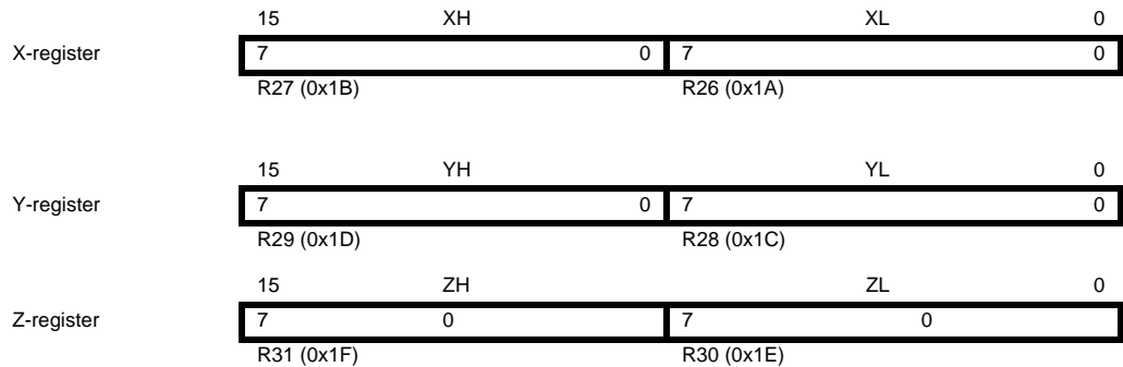
Figure 6-3. The X-, Y-, and Z-registers
