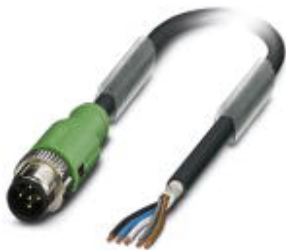
Sensor/actuator cable, 5-position, Variable cable type, shielded, Plug straight M12 SPEEDCON, A-coded, on free cable end, cable length: Free input (0.2 ... 40.0 m)
