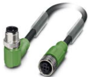
Sensor/actuator cable, 3-position, Variable cable type, shielded, Plug angled M12, A-coded, on Socket straight M12, A-coded, cable length: Free input (0.2 ... 40.0 m)
