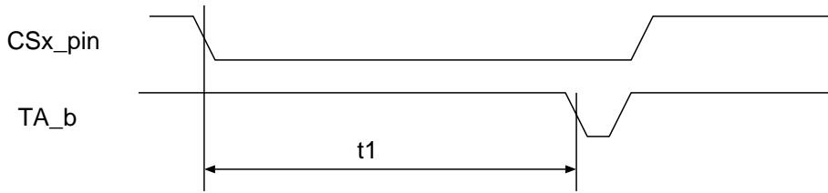
Figure 13-4 Non-IORDY Controlled IDE/SmartMedia TA Timing
