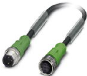
Sensor/actuator cable, 3-position, Variable cable type, Plug straight M12, A-coded, on Socket straight M12, A-coded, PIN 2+4 bridged, cable length: Free input (0.2 ... 40.0 m)
