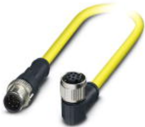
Sensor/Actuator cable, 8-position, PVC, yellow, Plug straight M12 SPEEDCON, A-coded, on Socket angled M12 SPEEDCON, A-coded, Cable length: 0.5 m
