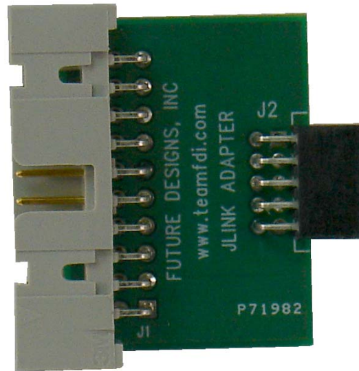
Figure 6 – FDI JTAG Adapter Board
