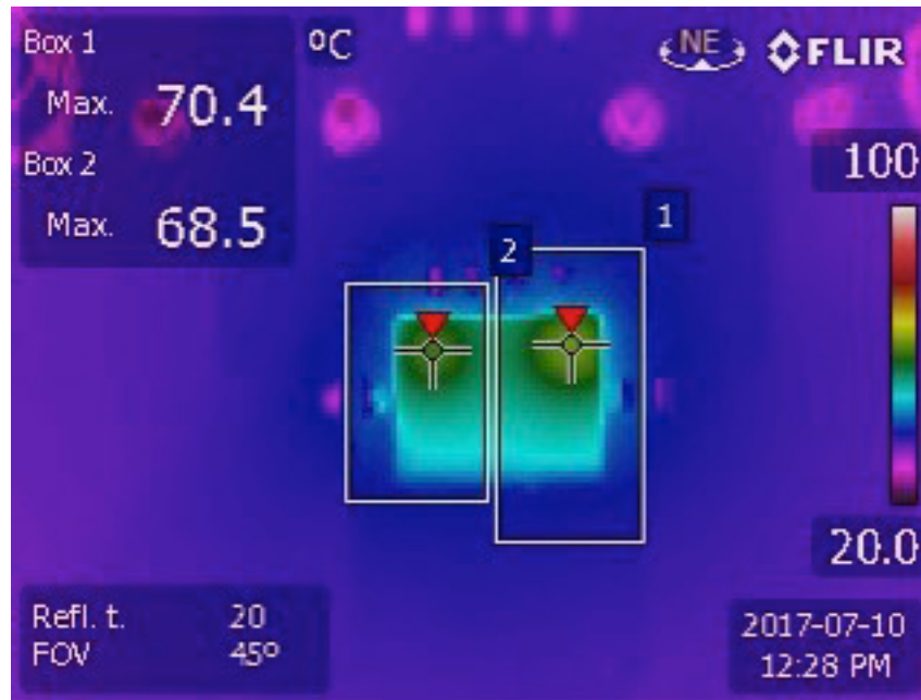
Figure 6. Thermal Image of LTM4646 V_{IN} = 12V , V_{OUT1} = 1.2V , I_{LOAD1} = 10A , V_{OUT2} = 1.5V , I_{LOAD2} = 10A Ambient Temperature = 25.0°C, No Forced Air Flow
