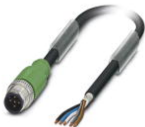
Sensor/actuator cable, 5-position, Variable cable type, shielded, Plug straight M12, A-coded, on free cable end, cable length: Free input (0.2 ... 40.0 m)
