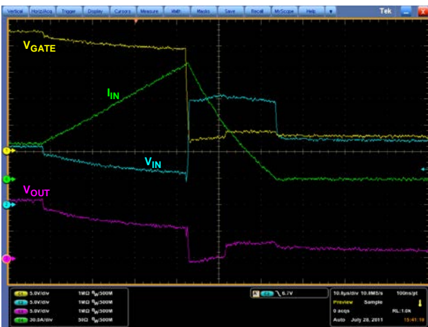
Figure 6. Output Short Circuit Zoom In
