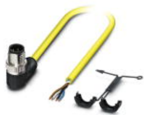
Sensor/Actuator cable, 4-position, PVC, yellow, Plug angled M12 SPEEDCON, A-coded, on free cable end, Cable length: 2 m
