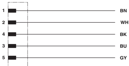
Contact assignment of the M12 plug
