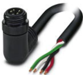
Power cable, 4-position, PVC, black, Plug angled 7/8"-16UNF, A - standard, on free cable end, A - standard, cable length: 2 m
