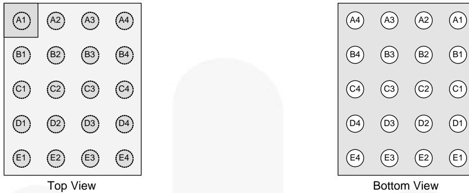
Figure 3. WLCSP-20 Pin Assignments
