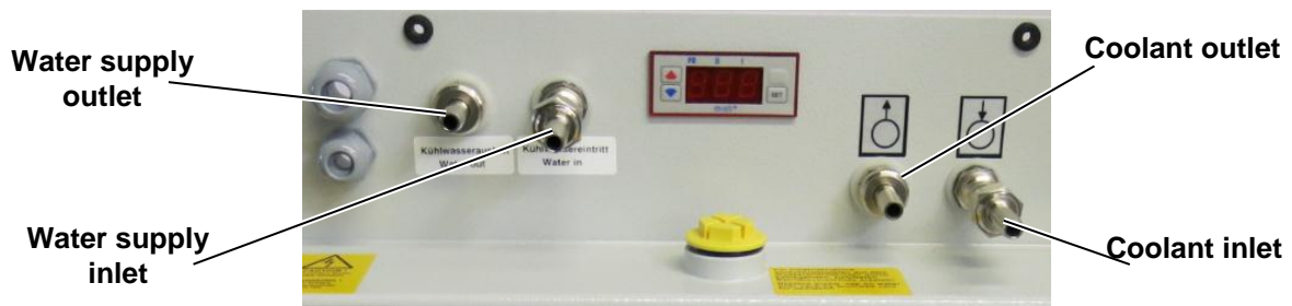
Fig. 8: Labelling of water inlet and water outlet
